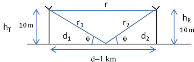
$$\psi = \text{atan} \left[ \frac{h_T}{d_1} \right] = \text{atan} \left[ \frac{h_R}{d_2} \right] \quad d = d_1 + d_2 = 10 \text{ km} \quad d_1 = d_2 = 500 \text{ m}$$
